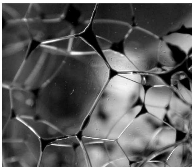
Fig. 9. The picture shows foam with thin Plateau borders and oil in the junction of the Plateau borders. The foam is from a foam test with 5 wt.% of oil e in synthetic sea water with 0.5 wt.% AOS content. The picture is taken 24 h after mixing and it is four times enlarged.
