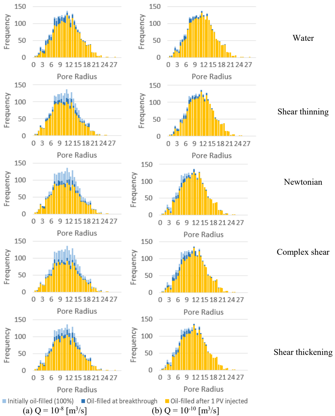
Figure 7.31: Oil filled bonds for the two cases (a) and (b). Light blue is the initial oil-filled bonds, dark blue is the oil-filled bonds at breakthrough, yellow is the oil left behind after 1 PV injected.
