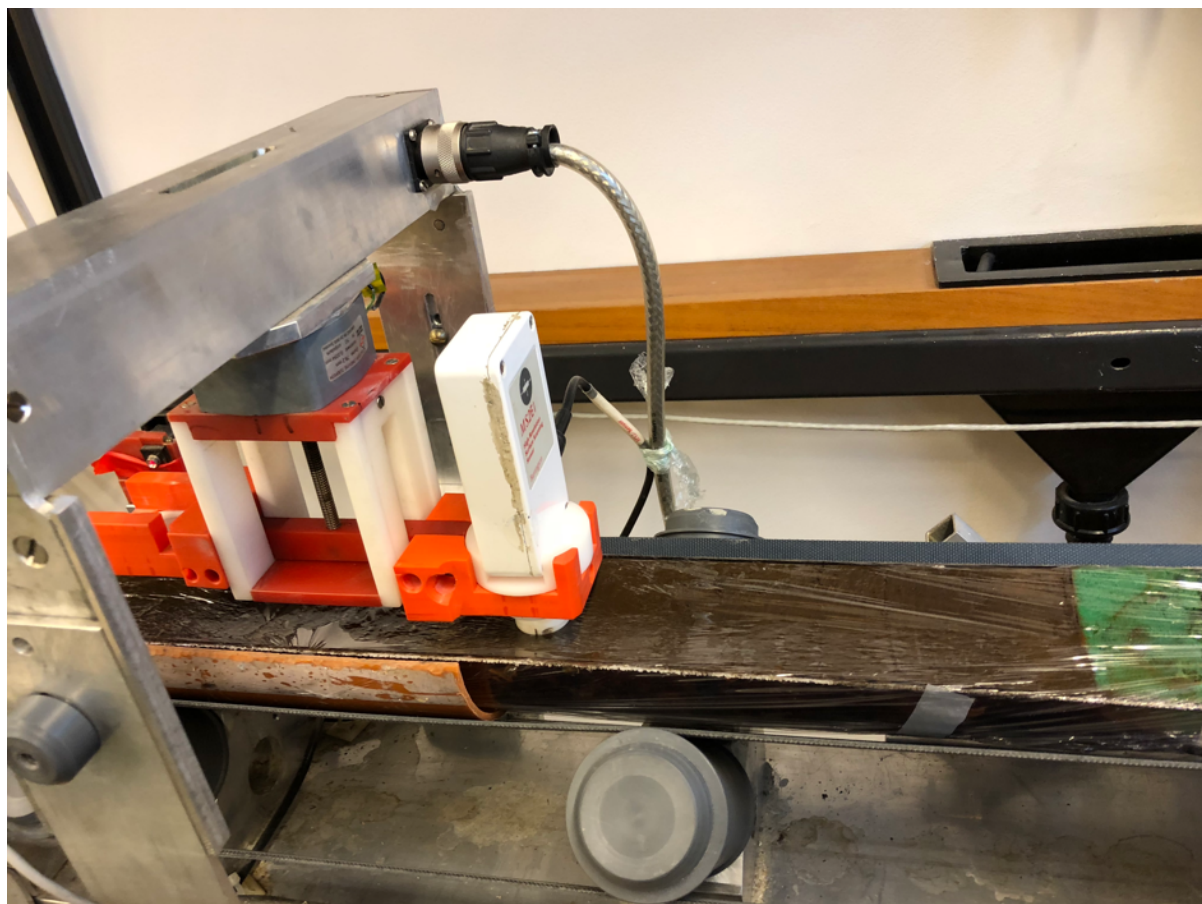
Figure 6: The point sensor moves up and down of contact with the core surface, which is an important factor when measuring magnetic susceptibility.
