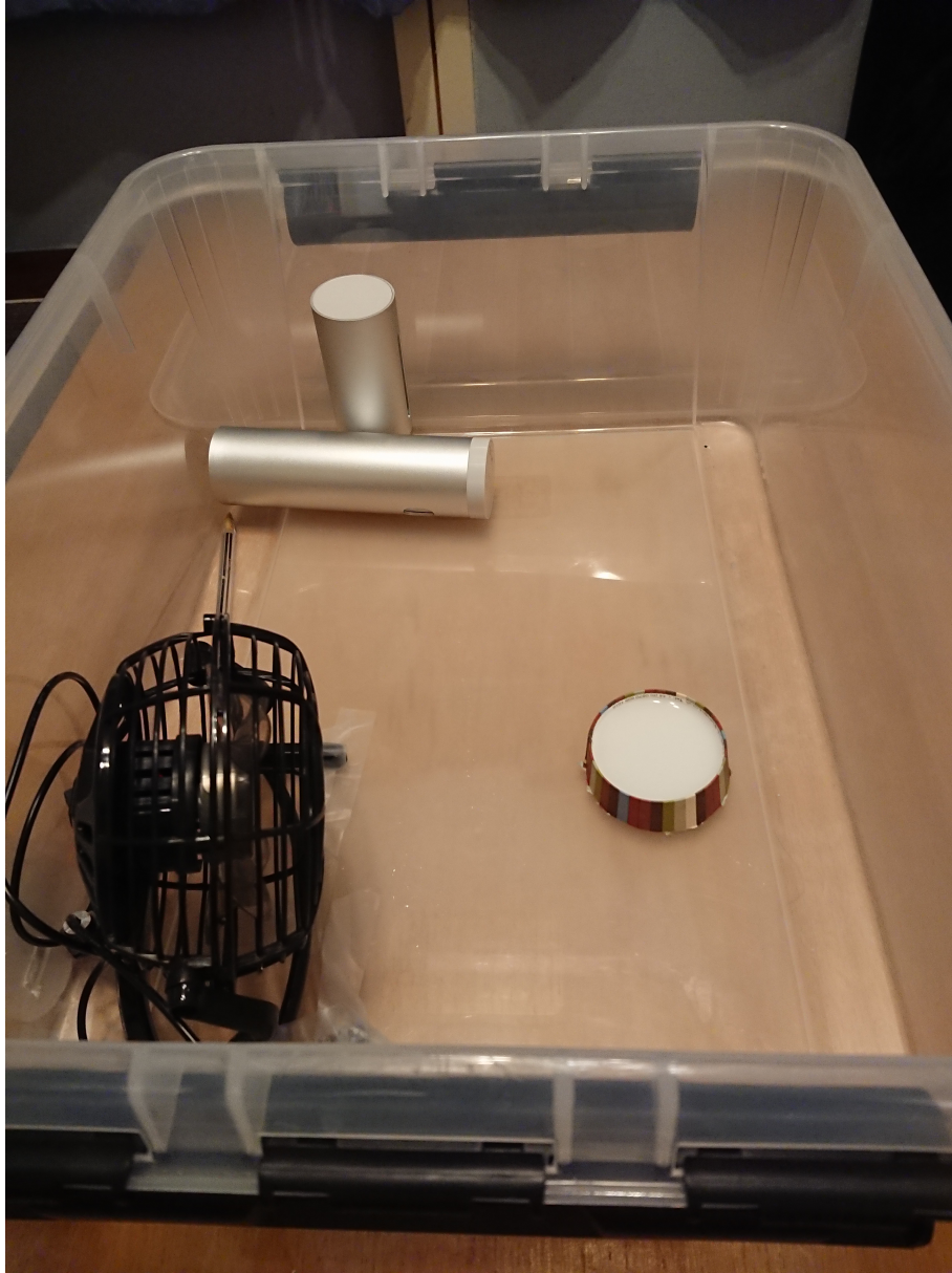
Figure 3.4: Plastic container used to create the controlled environment
