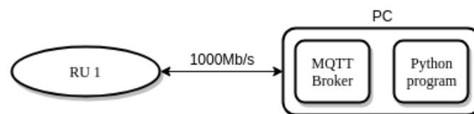
Figure 5.7: Request-response time test configuration.
