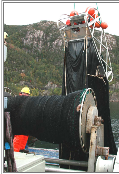
Figure 2 A pelagic midwater trawl with a multisampler attached
