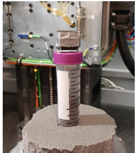
Figure 7 - Calibration cube placed on top of a synthetic minerogenic core containing basaltic tephra prior to scanning. Photo: Jan Magne Cederstrøm
