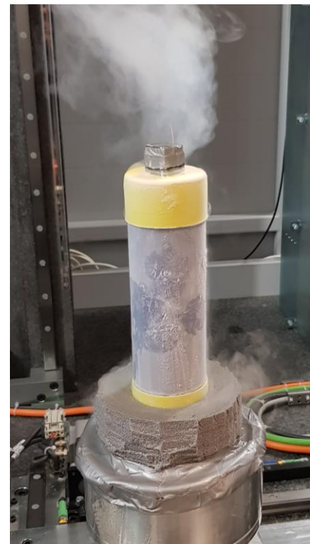
Figure 5 - Isolated plastic tube containing liquid nitrogen and the ice core with calibration cube placed on top inside the CT scanner. Photo: Jan Magne Cederstrøm
