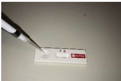
Figure 12 c. Eighty \mu L solution transferred to the Peptest device.
