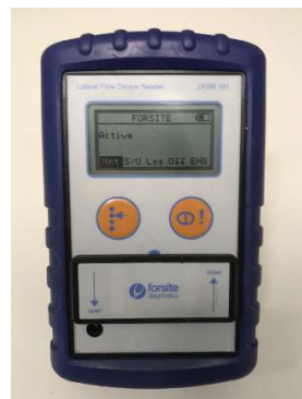
Figure 12 d. The LFDR-reader used for quantification of pepsin detected with the Peptest device.
