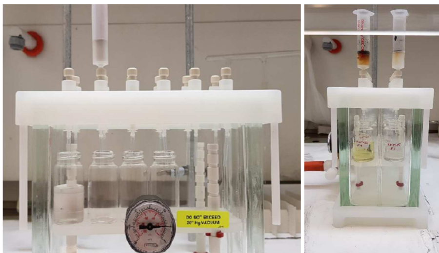
Figure 2.4. Supelco Visiprep™ apparatus together with the CN column used for Solid phase extraction of bio-oil samples.
