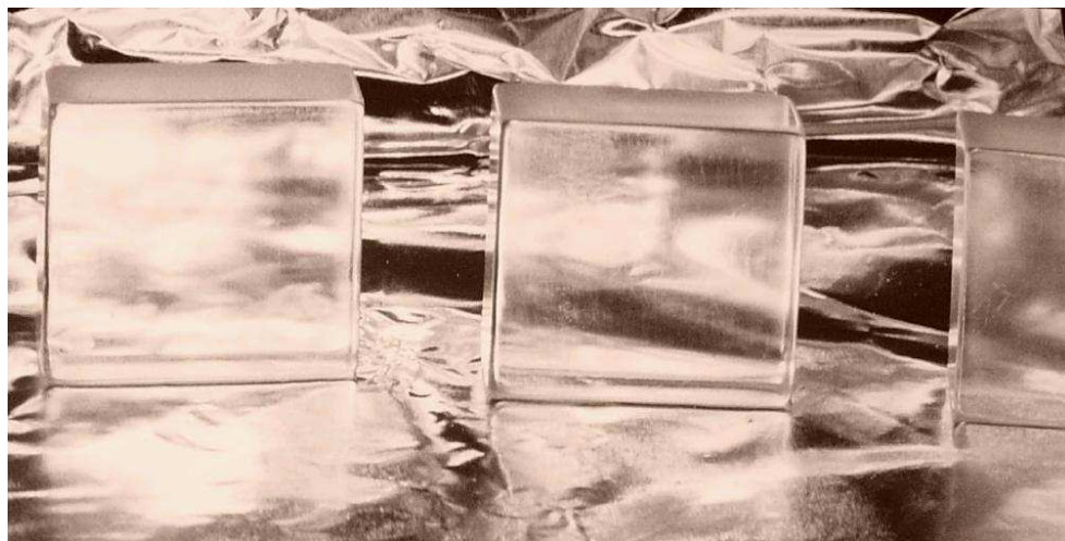
Figure A.2: New CsI(Tl) crystals in the process of being polished. The crystals are 4 \times 4 \times 1 \text{ cm}^3 blocks of scintillating material providing high photon yield for PIN-diode readout.
