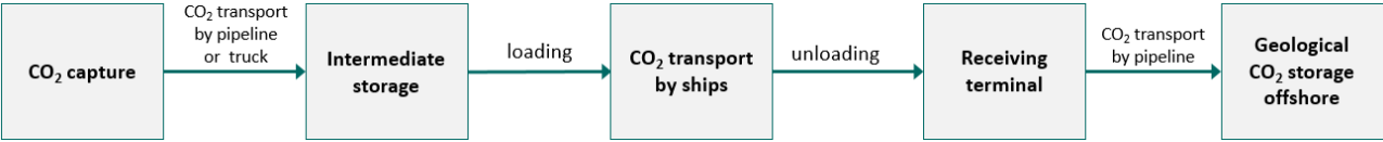
Figure 1: Planned CCS chain for the CCS demonstration project in Norway.
