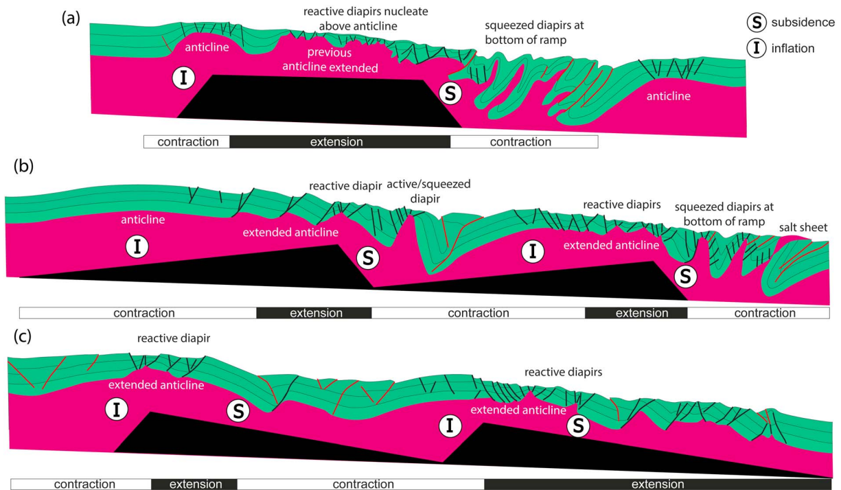
Figure 8. Synthesis diagram of final model results comparing structural style distribution associated with (a) a pre-salt horst, and pairs of tilted fault-blocks defined by (b) basinward-dipping and (c) landward-dipping pre-salt rift faults. (S) Indicates zones of subsidence and (I) zones of inflation and contraction. The distribution of structural domains is shown at the bottom of each section with extensional domains in black boxes and contractional domains in white boxes. Normal faults are shown in black and reverse faults in red. Pre-salt rift structures are in black, salt in pink and overburden in light green.
