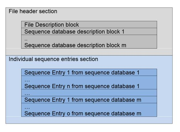
Figure 1. Overview of the PEFF schema. The file header section encodes metadata about the file itself and about the one or more sequence databases contained in the file. The individual sequence entries section encodes each of the individual sequences and the metadata associated with each entry.
