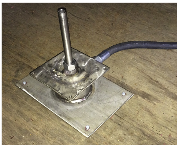
Fig. 12. Pipe used for vertical jet release.
