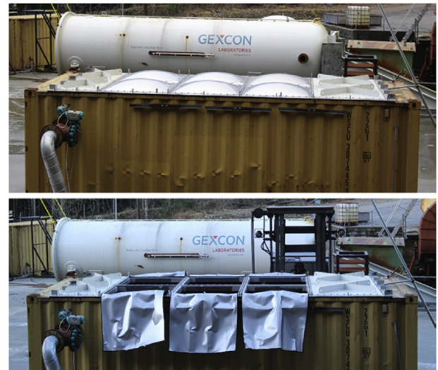
Fig. 6. Container with six commercial vent panels before and after a test.
