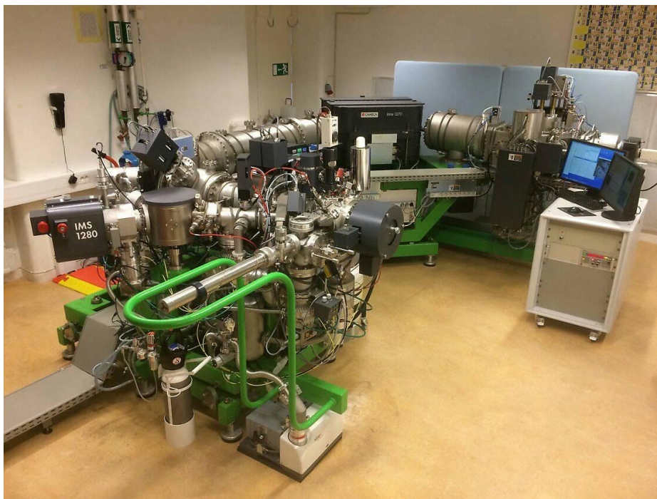
Figure 4.4: CAMECA IMS1280 ion microprobe used to generate U–Th–Pb analysis for the picked zircons. Nordsim facility in Stockholm. Photo: Cheng–Cheng Wang.
