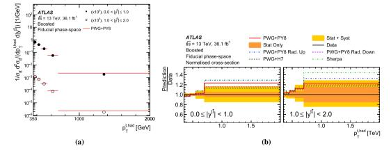
**Fig. 44** a Particle-level normalised differential cross-section as a function of  $p_{\rm T}^{t,{\rm had}}$  in bins of the absolute value of the rapidity of the  $t\bar{t}$  system in the boosted topology compared with the prediction obtained with the POWHEG+PYTHIA8 MC generator.Data points are placed at the cen-
