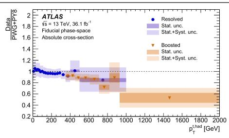
Fig. 54 The ratios of the measured fiducial phase-space absolute differential cross-sections to the predictions obtained with the POWHEG+PYTHIA8 MC generator in the resolved and boosted topolo-
