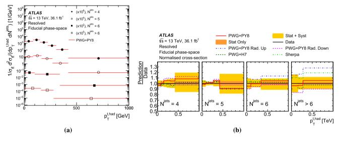
Fig. 29 a Particle-level normalised differential cross-section as a function of  $p_{\rm T}^{t,{\rm had}}$  in bins of the jet multiplicity in the resolved topology compared with the prediction obtained with the POWHEG+PYTHIA8 MC
