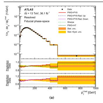
Fig. 22 Particle-level normalised differential cross-sections as a function of **a** the transverse momentum and **b** the absolute value of the rapidity of the hadronically decaying top quark in the resolved topology, compared with different Monte Carlo predictions. The bands rep-
