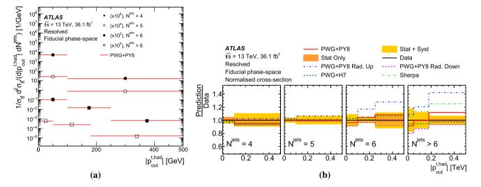
**Fig. 33** a Particle-level normalised differential cross-section as a function of  $\left| p_{\text{out}}^{t,\text{had}} \right|$  in bins of the jet multiplicity in the resolved topology compared with the prediction obtained with the POWHEG+PYTHIA8 MC
