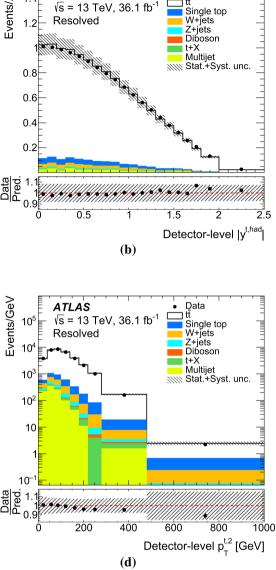
Fig. 6 Distributions of observables in the  $\ell$ +jets channel reconstructed with the pseudo-top algorithm in the resolved topology at detector-level: **a** transverse momentum and **b** absolute value of the rapidity of the hadronic top quark, **c** transverse momentum of the leading top quark and **d** transverse momentum of the subleading top quark. Data distributions are compared with predictions, using POWHEG+PYTHIA8 as the  $t\bar{t}$
