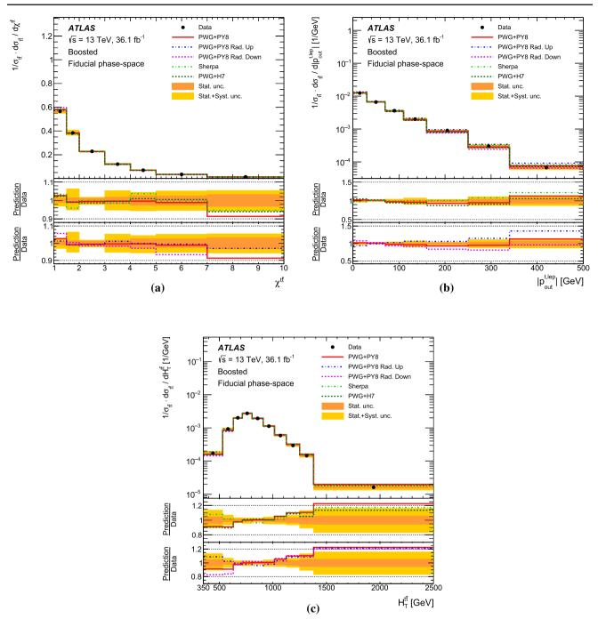
**Fig. 41** Particle-level normalised differential cross-sections as a function of **a**  $\chi^{t\bar{t}}$ , **b**  $|p_{out}^{t,lep}|$  and **c**  $H_{T}^{t\bar{t}}$  in the boosted topology, compared with different Monte Carlo predictions. The bands represent the statisti-
