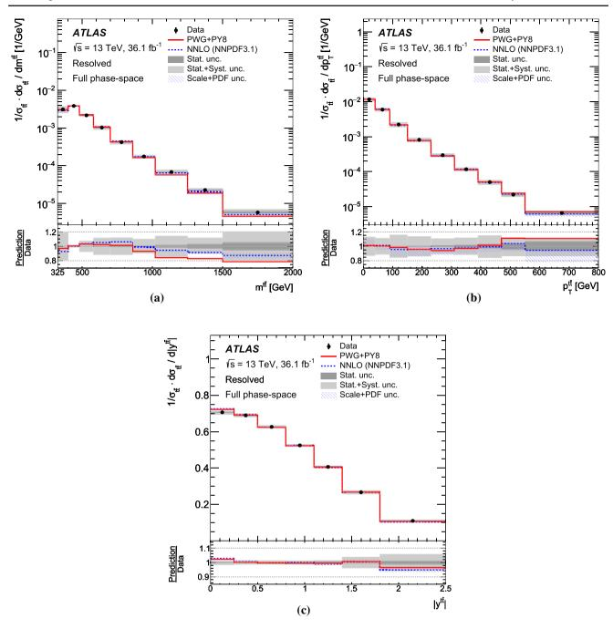
Fig. 56 Parton-level normalised differential cross-sections as a function of **a** the mass, **b**  $p_{\rm T}$  and **c** absolute value of the rapidity of the  $t\bar{t}$  system in the resolved topology, compared with the NNLO predictions obtained using the NNPDF3.1 NNLO PDF set and the predictions obtained with the POWHEG+PYTHIA8 MC generator. The hatched band
