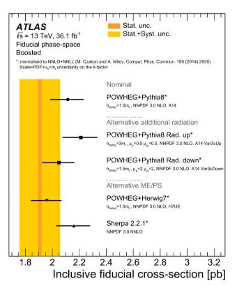
**Fig. 53** Comparison of the measured inclusive fiducial cross-section in the boosted topology with the predictions from several MC generators. The bands represent the statistical and total uncertainty in the data.
