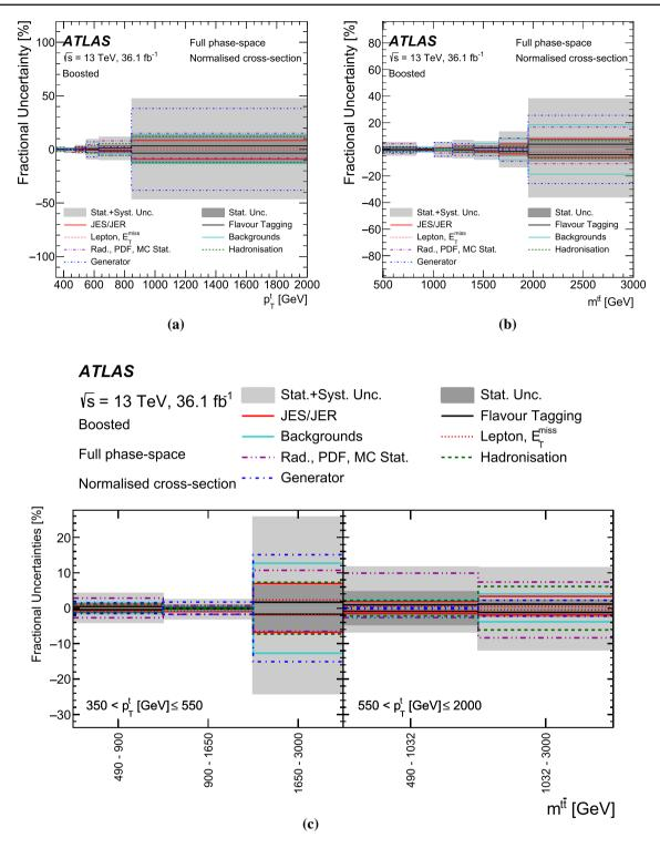
Fig. 21 Uncertainties in the parton-level normalised differential crosssections as a function of **a** the transverse momentum of the top quark, **b** the mass of the  $t\bar{t}$  system and **c** the mass of the  $t\bar{t}$  system as a function
