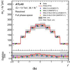
Fig. 64 Parton-level absolute differential cross-sections as a function of a  $p_T^t$  and b  $y^t$  in the resolved topology. The results are compared with NNLO QCD and NNLO QCD+NLO EW theoretical calculations using the NNPDF3.1 and LUXQED17 PDF sets. The vertical bars on each marker represents the total uncertainty in the prediction. The solid
