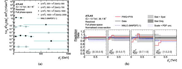
**Fig. 60** a Parton-level normalised differential cross-section as a function of  $p_{\rm T}^t$  in bins of  $m^{t\bar{t}}$  in the resolved topology compared with the NNLO prediction obtained using the NNPDF3.1 NNLO PDF set. Data points are placed at the centre of each bin. **b** The ratio of the measured
