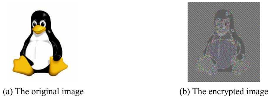
Figure 4.1: Image encrypted using ECB mode
