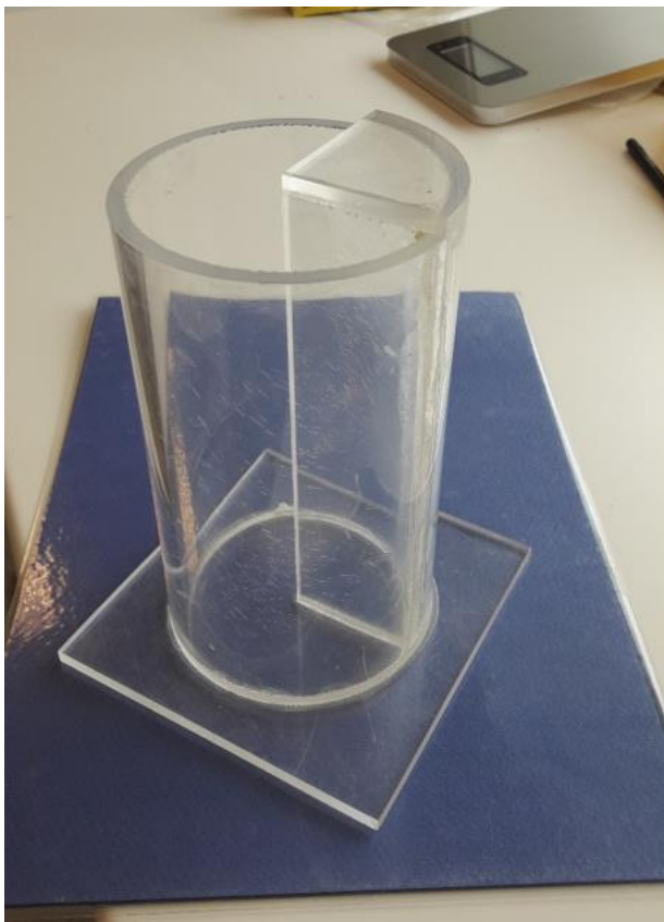
Figure 2.1: The plankton splitter that has been used for splitting samples. The cylinder part has an outer diameter of 9 centimetres and a height of 15 centimetres, giving it a total volume of 0.95 litres. All sides of the rectangle are 12 cm.
