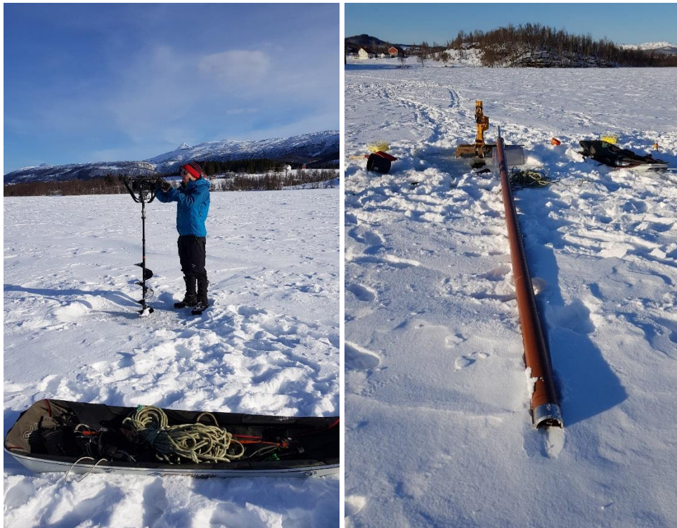
Figure 3.4: Lake Coring with piston corer (Photo: Kristian Vasskog).
