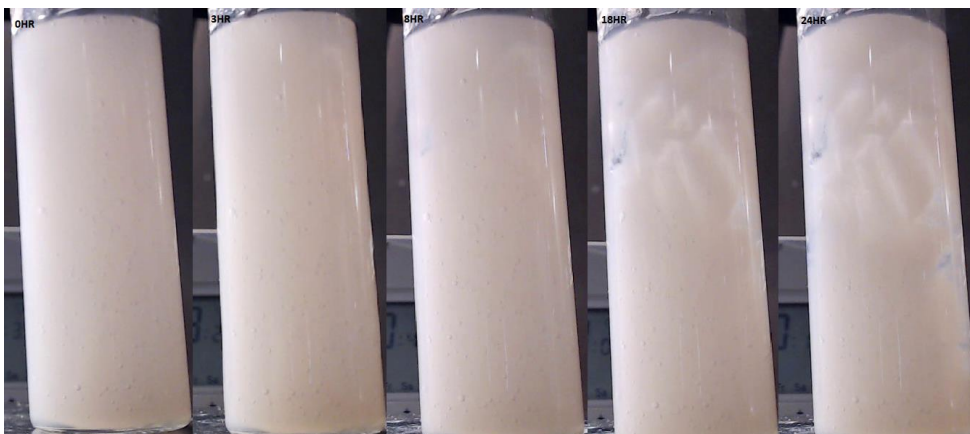
Figure 4-5: Hydrate growth of sample 0.3µm-D-NC-1 over a 24-hour period.
