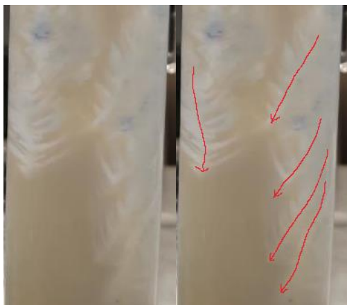
Figure 5-3: Close-up of sample 0,3 \mu m-D-NC-2 24 hours after nucleation. The red arrows highlight where the veins sprout downwards throughout the sample.
