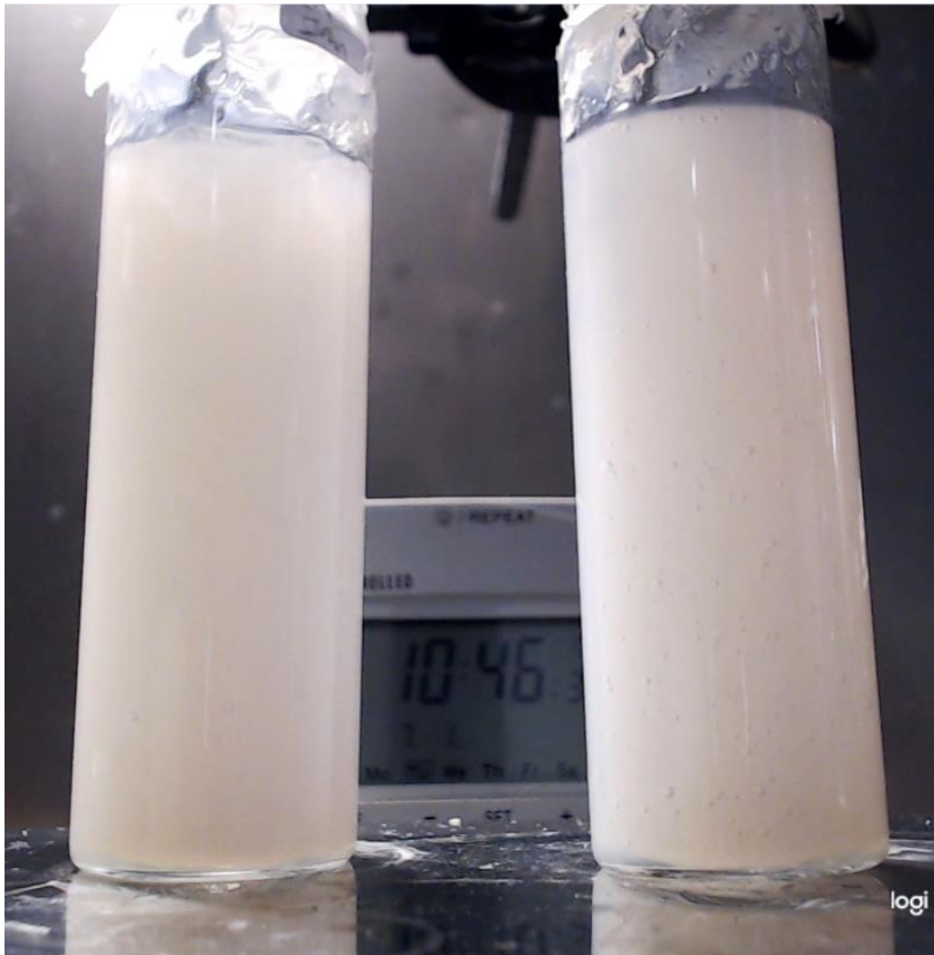
Figure 3-1: Experimental set-up used for the first samples 11 as seen through the web camera. Two samples are recorded simultaneously. A PT-100 temperature sensor is submerged into the sample from the top, and parafilm is used to seal it.
