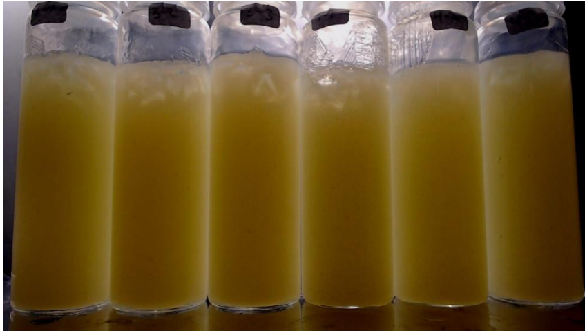
Figure 4-11: Samples from left to right; 12nm-D-C-1, -2, -3 and 0,3 \mu m-D-C-1, -2, -3. This figure shows the samples three hours after nucleation by ice seeding.
