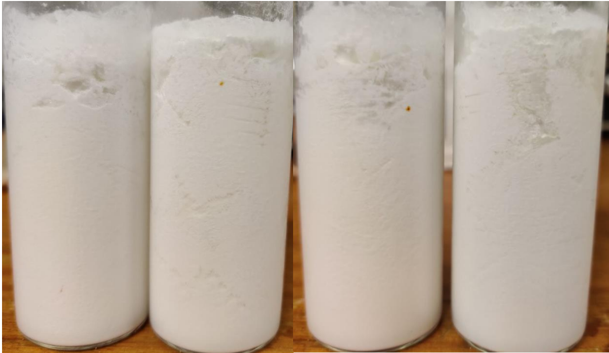
Figure 4-29: M5-D-C-1 and M5-D-C-2 frontside (left) and rear (right) 48 hours after nucleation. The two yellow specks visible are tiny undissolved agglomerates of colouring. Some frost build-up is observed on the glass in the front of sample M5-D-C-1 and the rear of sample M5-D-C-2.
