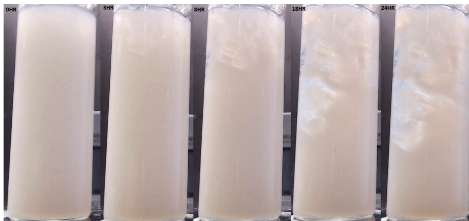
Figure 4-1: Hydrate growth of sample 12nm-D-NC-1 over a 24-hour period.
