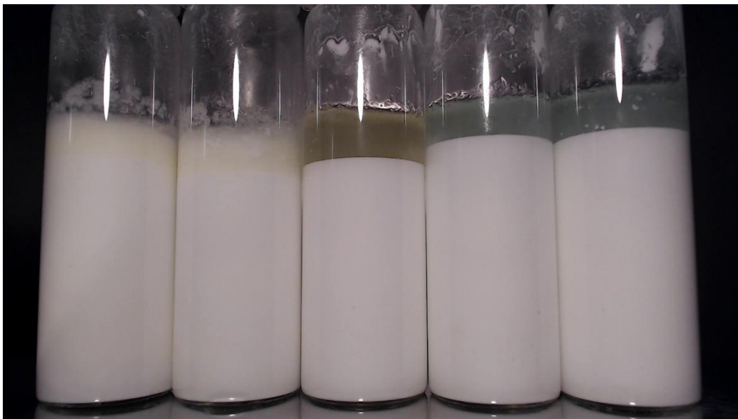
Figure 4-32: Ice seeding at 0 hours. Samples from left to right: M5-D-C-3, -4, M5-3,5%-C-3, M5-U-C-3, -4. The cloudiness of the liquid above sample M5-D-C-3 and M5-D-C-4 stems from the suspension of silt present in Micro5 quartz sand when handling the samples.
