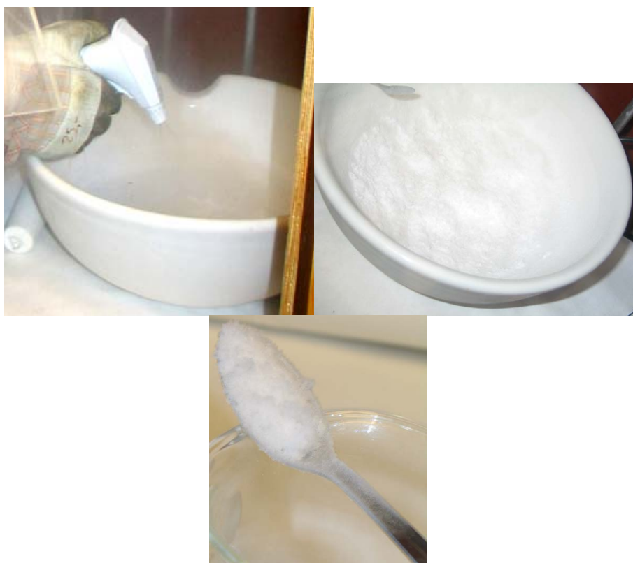
Figure 1: Tiny ice crystals are made by spraying water into liquid nitrogen.
