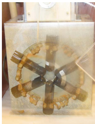
Figure 3: The oil samples were run in a rotating wheel for three days.
