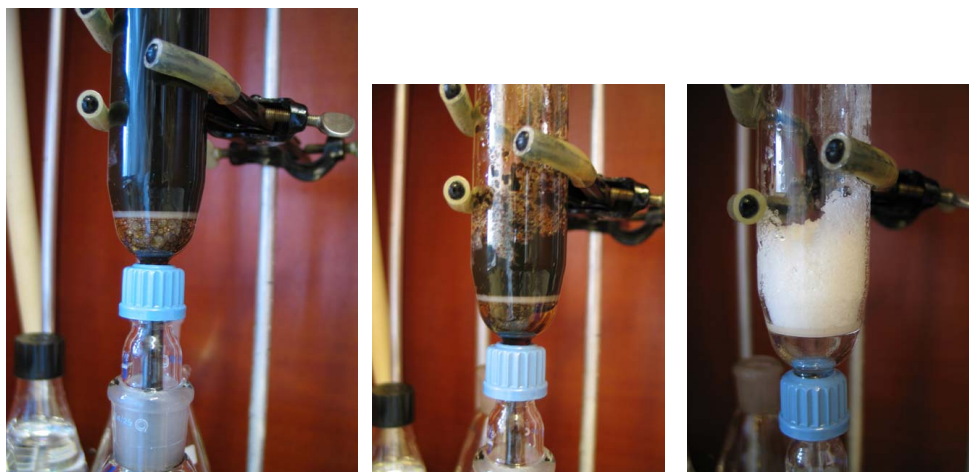
Figure 4: Ice extraction by the use of a column packed with ice. Left: Ice and oil in the column. Middle: The oil has passed through the ice. Right: The ice is washed with toluene to remove excess oil.
