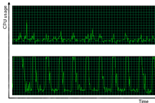
Fig. 16. CPU consumption of the MoPS project PC during barrel cosmics run. The plot shows regular peaks at 100% with a period corresponding to the MoPS reading rate (15 seconds).
