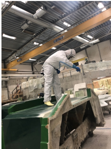
Picture 11. Gel coating with gun-spray [31]
