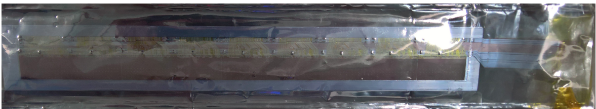
Figure 3.1: A prototype 9 chip string fixed to an aluminium backing plate and covered in anti static protection.
