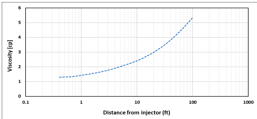
Figure 12. Viscosity profile after injecting 1 PV at 5000 bbl/day for shear thinning rheology.
