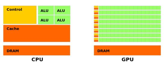
Figure 3.1: CPU vs GPU [48]
