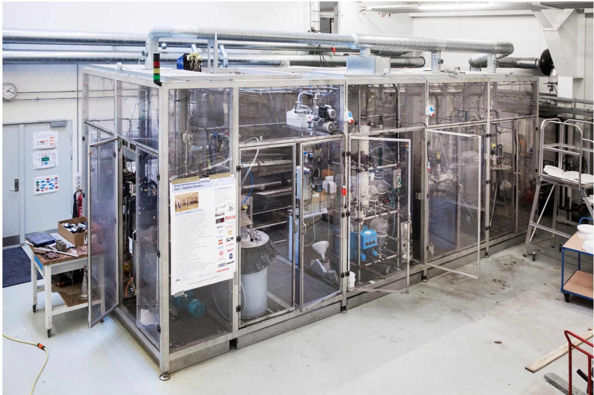
Figure 1.1: Photo of the continuous flow pilot-scale HTL reactor placed at the Center for Biorefining Technologies (CBT) in Foulum, and belonging to Aarhus University.
