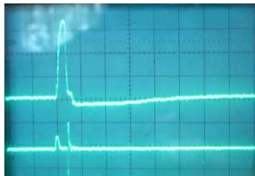
Figure 3.6f: The pulse-signal at spark discharge.
