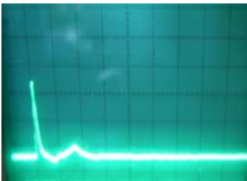
Figure 3.6c: The pulse signal from amplifier A2. The first peak has a voltage value of about 90 V and the second of about 19V.
