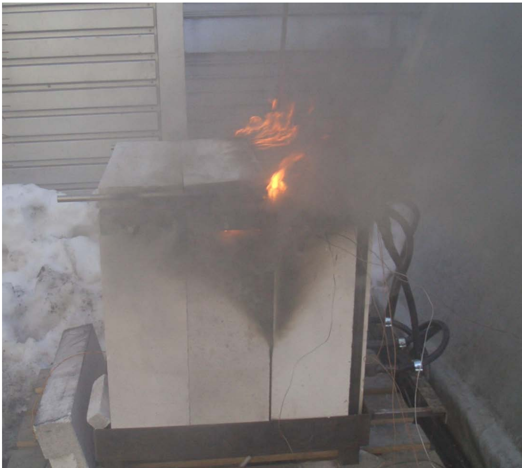
Picture 13 shows the furnace during experiment 050309. Flame tongues are visible around the air gap.
