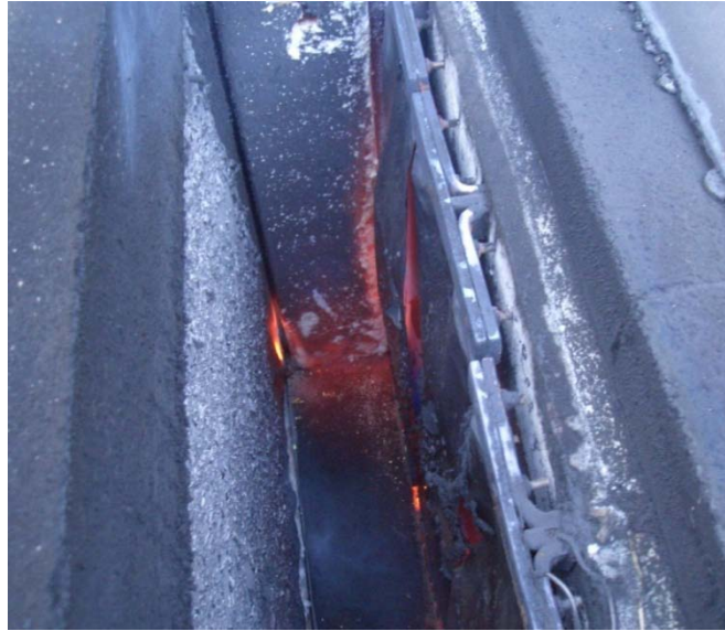
Picture 18 shows the furnace from the inside right after experiment 060309_02 was performed. There are still visible flames inside the furnace, both behind the foils and behind the isolation on the edges.
