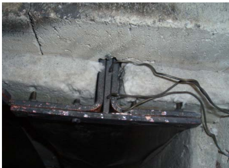
Picture 8 to the left shows one of the copper plates with all the thermocouples in place.
