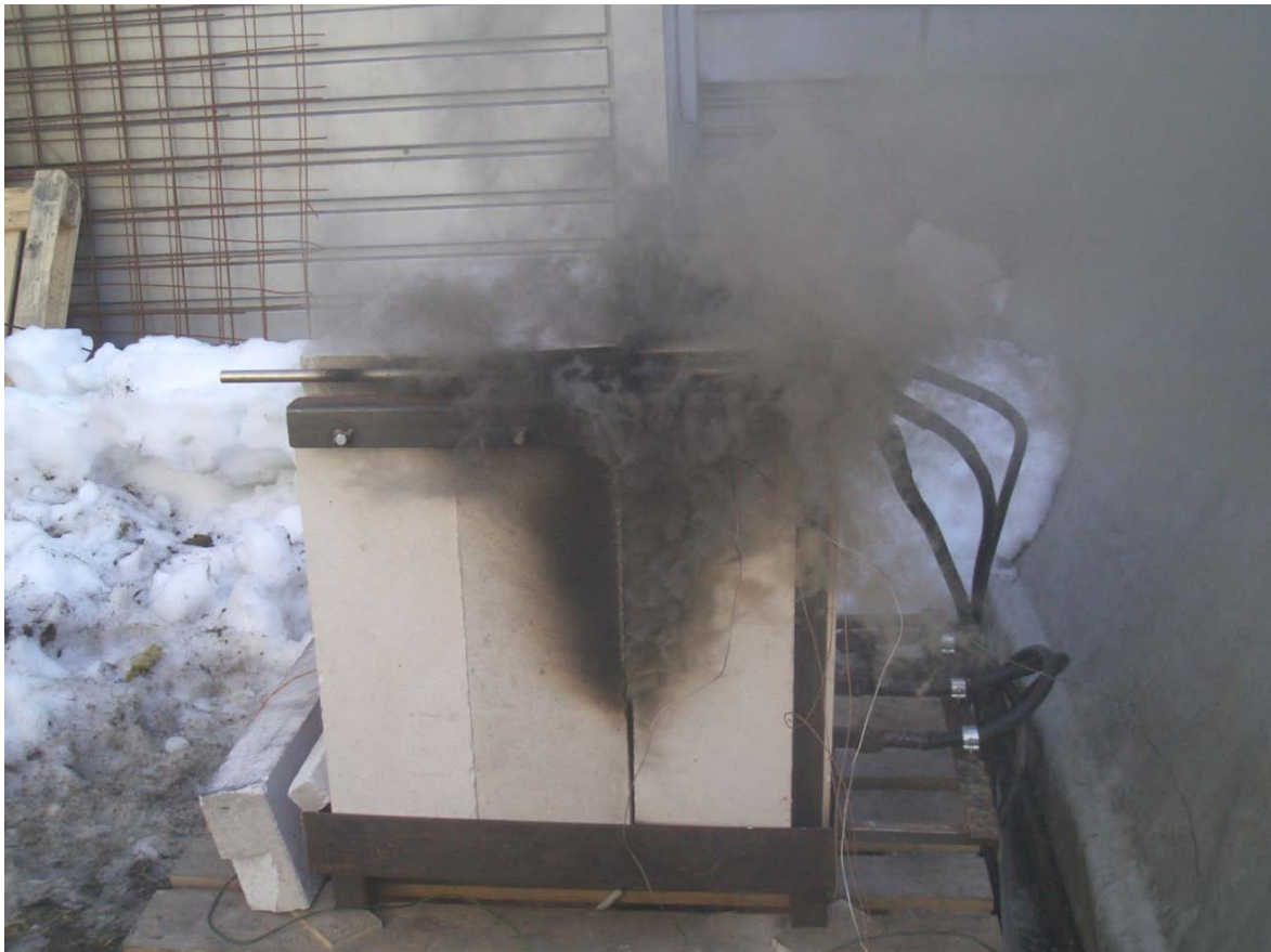
Picture 15 shows the furnace during experiment 050309. No flame tongues are visual, but the specimen still produces a lot of smoke.
