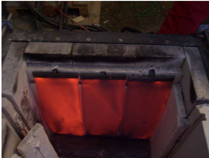
Picture 3 shows the radiation foils when the power supply is switched on.
