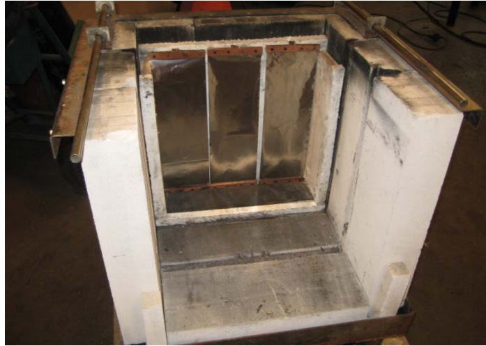
Picture 2 shows how the testing furnace looks like inside without any test specimen. Three vertical foils are shown in this picture that function as the radiation panel.
