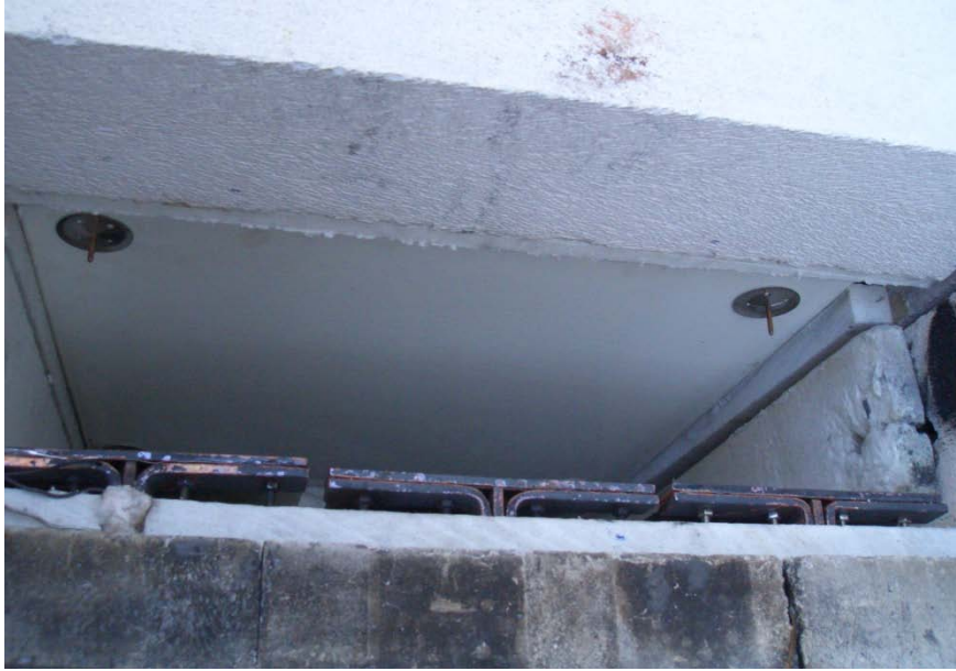
Picture 10 shows ProTek B3 (an intumescent material) ready to be tested inside the furnace.
