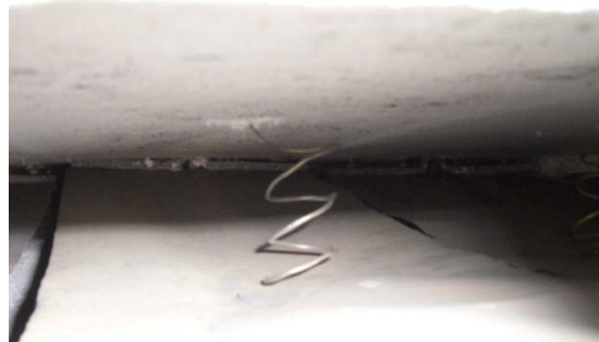
Picture 6 shows how the surface temperatures on the foils were measured in the experiments 181108 to 041208.
