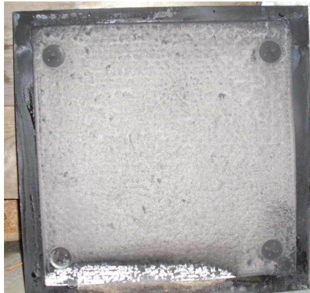
Picture 11 shows ProTek B3 (an intumescent material) fastened to a steel plate after being exposed to heat for about an hour
