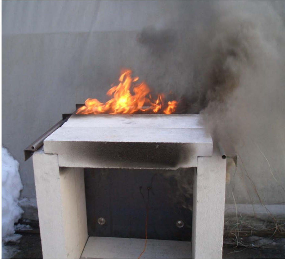
Picture 14 shows the furnace during experiment 050309. Flame tongues are visual around the air gap.
