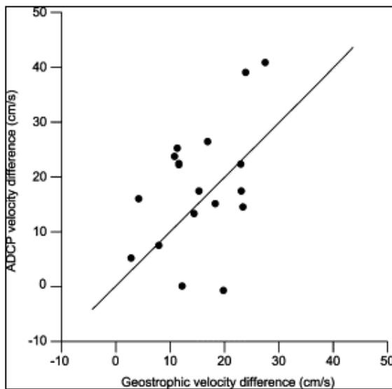
Fig. 13. Eastward velocity difference (shear) between 200 and 500 m depth measured by ADCP (daily average) at site NB compared to geostrophic shear between the same levels calculated from CTD observations at stations N04 and N05 on the same day. The line indicates equality.
