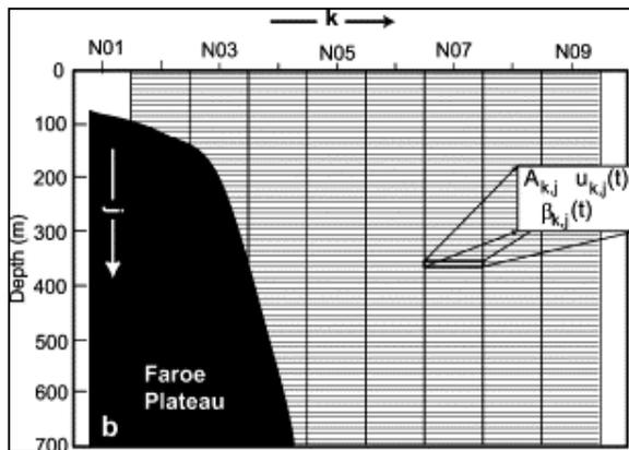
Fig. 16. Subdivision of section N into boxes for calculating fluxes. Boxes are labeled by indices  $k$  and  $j$ . One of the boxes is shown in a magnified scale indicating the parameters that must be assigned to each box: the area:  $A_{k,j}$ , the eastward velocity:  $u_{k,j}(t)$ , and the fraction of Atlantic water:  $\beta_{k,j}(t)$ .
