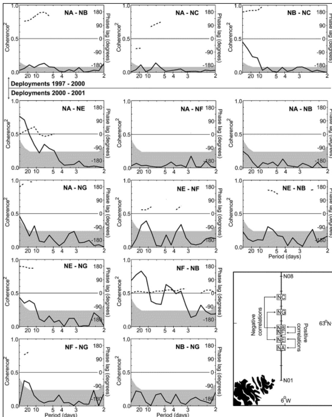
Fig. 15. Squared coherence (thick continuous curves) and phase lags (dashed curves) for pairs of eastward velocity time series (average 0–200 m) from deployments on section N. The coherence spectra were estimated using MATLAB with linear de-trending and Hanning windows with 50% overlap. In each graph, the shaded area indicates non-significance at the 99% level estimated by 10,000 Monte Carlo simulations of pairs of white noise series. Phase lag is
