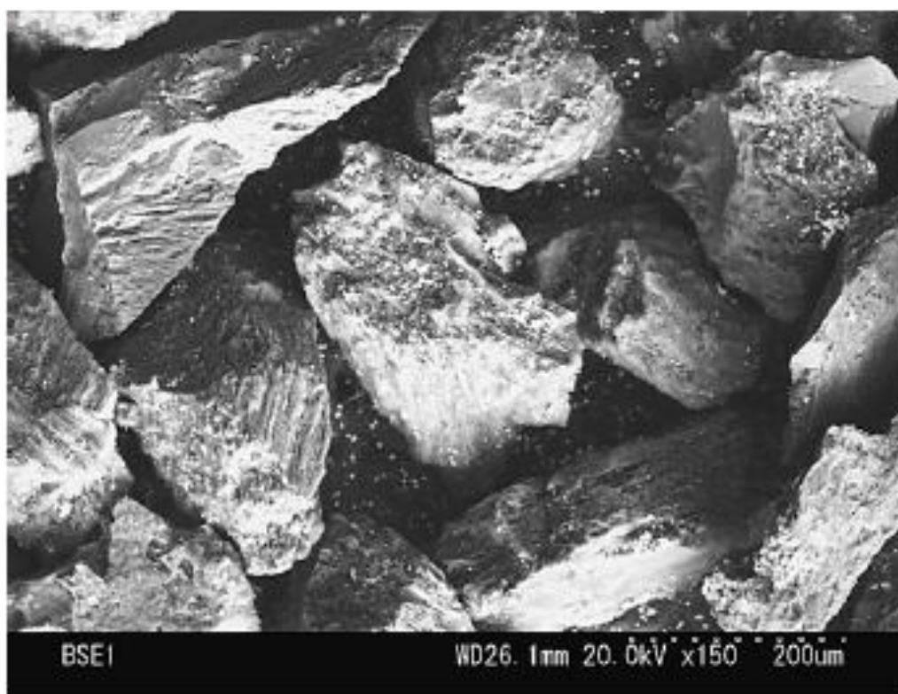
Figure 5-1: Electron microscope picture of granulated activated carbon.
