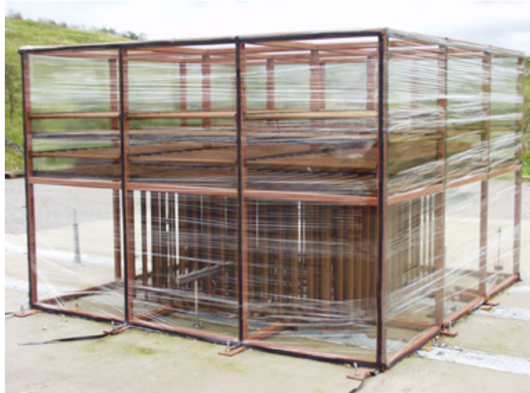
Figure 5.10 – A picture of the congestion rig with plastic film (Royle, Shirvill & Roberts, 2007).
