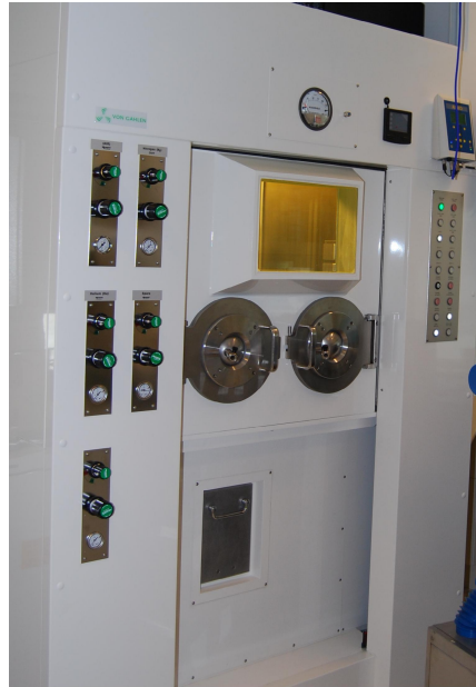
Figure 5.8: The front of the hot cell. With lead window and circular holes for the hands.
