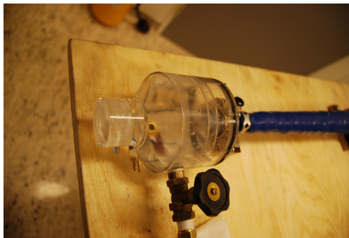
Figure 5.7: Image of the particle box, the blue is the lower end of the hydrocyclone, and valve for controlling underflow. Bottom hole is for draining of particle box.
