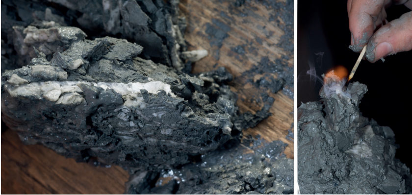
Figure 6.1: Natural gas hydrate from the G11 pockmark at Nyegga just after recovery.
