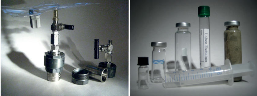
Figure 5.2: To the right the autoclave used for hydrate sampling and containing is displayed. The left hand picture show a cut syringe used for sediment sampling and five sampling vials. From the left; pore water for VOA, pore water for headspace, sediment headspace samples, gas container for isotope analysis and a example of a interstitial sediment sample stirred with 1 ml NaOH.
