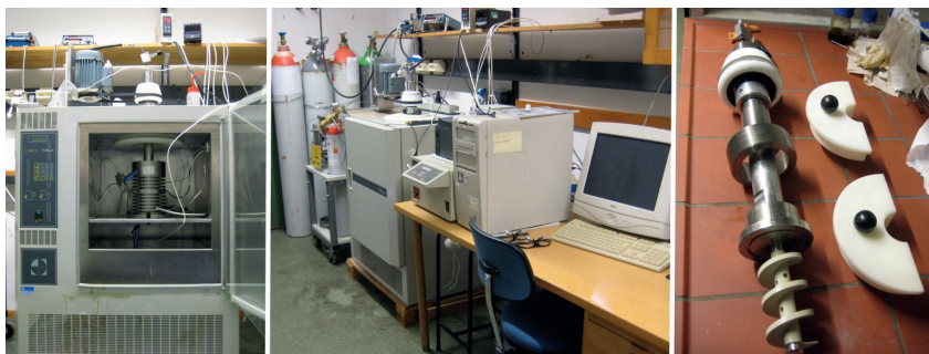
Figure 5.3: Left; the hydrate cell inside the heating cabinet and torque stirring system integrated through the top. Middle; the incubator shown in connection to gas supply and computer monitoring. Right; the hard shaft with the torque screw.
