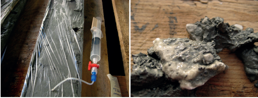
Figure 5.1: The left picture shows pore water extraction with a Rhizon syringe system. To the right, natural gas hydrate recovered during the GS08-155 Cruise, from the G11 pockmark at Nyegga, is dissociating on deck.
