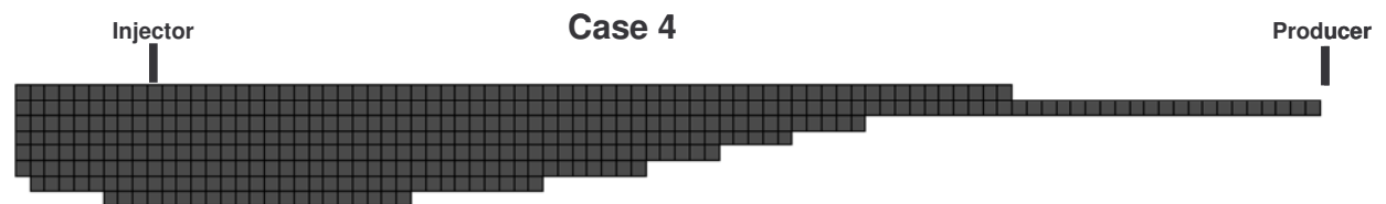
Fig. 9: Three-phase zone case 4: three-phase relative permeability hysteresis and trapping including capillary pressure.
