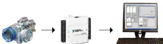
Figure 3.4.5: Chart of data acquisition circuit; Differential pressure transmitter – Voltmeter – LabVIEW program.
