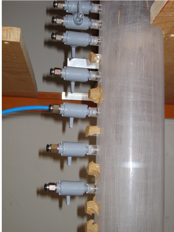
Figure 4.6: The pressure tapings on the separator body.
