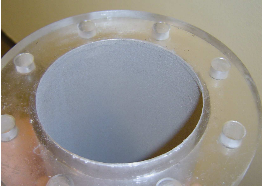
Figure 4.7: The separator tube covered with metal particles.
