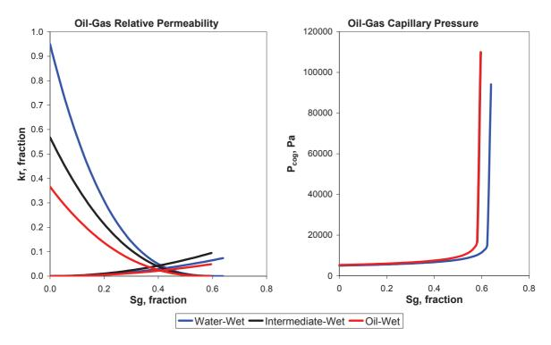
*Figure 2. Smoothed two-phase oil-gas relative permeability and capillary pressure from network model for different wettability system*
