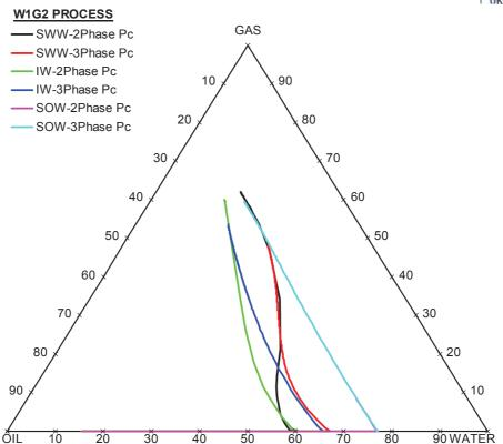
Figure 10. Saturation path at block (2,2,1) for different wettability system, W1G2 process, using twophase and three-phase capillary pressure
