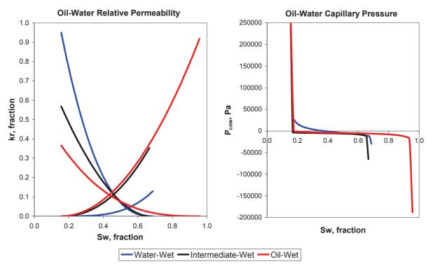
*Figure 1. Smoothed two-phase oil-water relative permeability and capillary pressure from network model for different wettability system*
