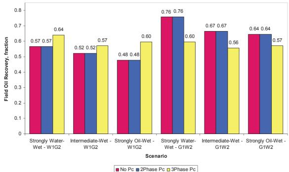
Figure 7. Field oil recovery at the end of simulation
