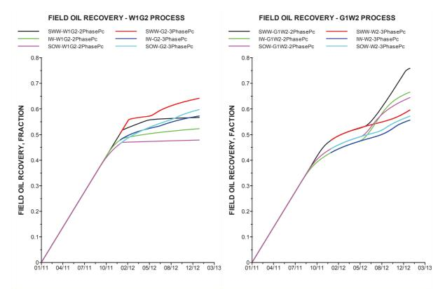
Figure 6. Recovery efficiency for different wettability system and different process, with two-phase and three-phase capillary pressure
