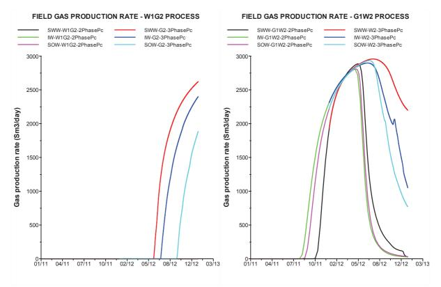
Figure 9. Gas production rate profile for different wettability system and different processes, with two-phase and three-phase capillary pressure
