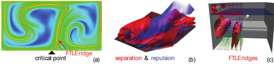
Figure 5: Applications of FTLE to visualization. (a) In the double gyre example the critical point is disjunct to the FTLE ridge separating different regimes of the flow (image created following Shadden et al. [185]). (b) Volume rendering of the FTLE field shows the regions of locally maximally attracting and repelling behavior (image courtesy of Garth et al. [42] © 2007 IEEE). (c) Extraction of ridges from the FTLE field allows additional processing and filtering to concentrate on the salient features of the flow (image courtesy of Sadlo et al. [168] © 2007 IEEE).
