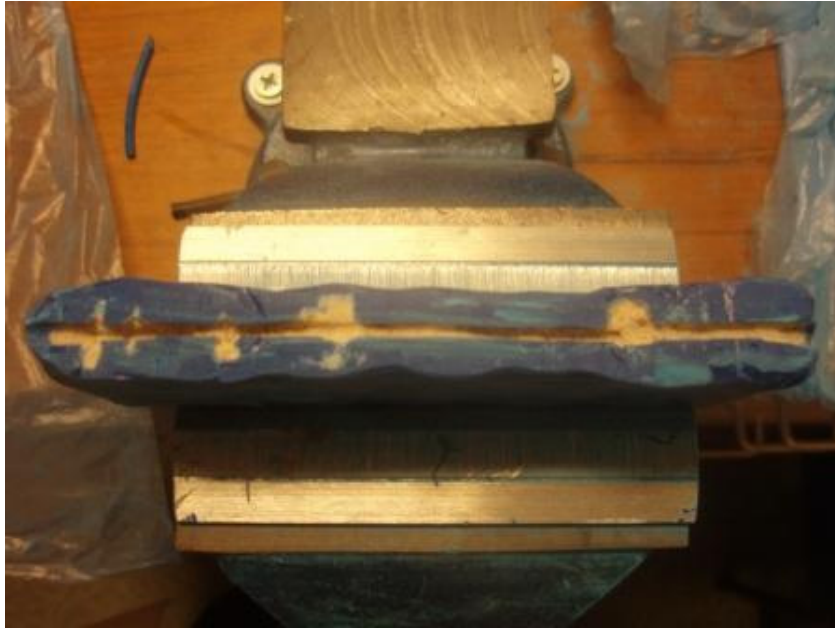
Figure 4-5: Sample A', under preparation (epoxy coating).
