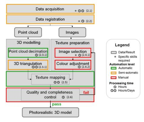
Figure 2.1. Workflow for creation of textured photorealistic 3D models (modified after Buckley et al. (2008a)).
