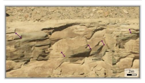
Figure 2.3. Texture artefacts (darker patches) caused by registration errors and imperfect implementation of additional camera calibration parameters in areas covered by multiple images. Texture displacement marked in purple.
