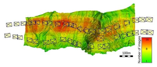
Figure 2.2. 3D terrain model and footprints (navy blue polyhedrons) of acquired images, a section of the Book Cliffs, Utah, USA. Mesh triangles coloured depending on the number of covering images. Output from method presented in this thesis (Paper A).
