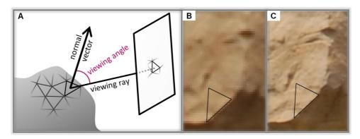
Figure 2.4. Camera – triangle viewing angle (A). Low (B) and high (C) effective triangle resolution within the image.
