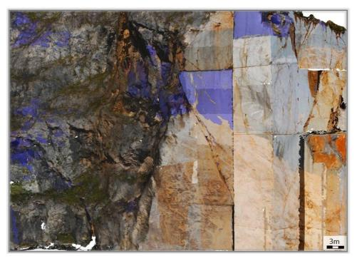
Figure 1.2. 3D outcrop model textured with RGB images and results of hyperspectral classification. Limestone patches marked in blue.
