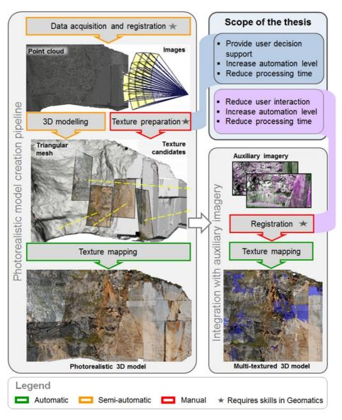
Figure 1.3. General workflow for creation of photorealistic 3D models and integration with auxiliary image data, with a highlight of the two areas addressed in this thesis.
