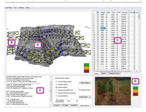
Figure 4.1. Framework for visualisation and analysis of texture parameters. The 3D scene is composed of a 3D model (A) and footprints of the overlapping images (B). Numerical image quality indicators are reported in a table (C) and as a colour-coded map (here: the viewing angle) overlaid on the original image thumbnail (D). Numerical texture quality indicators are reported in a log window (E).
