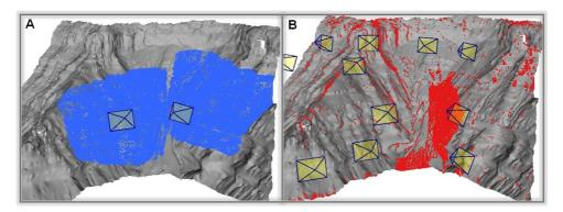
Figure 4.3. Two ways to control texture completeness: by highlighting image ground coverage (A), and by highlighting triangles not covered (without texture) by an image subset (B).
