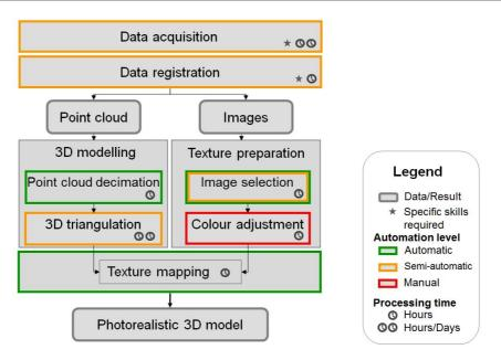
Figure 4.4. Improved workflow for creation of virtual outcrop models.
