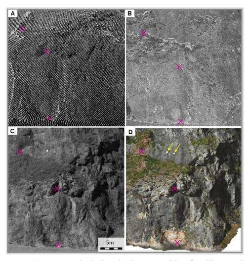
Figure 3.2. Laser point cloud coloured with intensity of the reflected laser signal (A), and the corresponding part of: the 2D image created from intensity values (B), the hyperspectral scan, band 1.336µm (C), and the 3D model textured with RGB images (D). Purple crosses mark homologous points in datasets. Reflective targets marked with yellow arrows.
