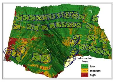
Figure 4.2. 3D model coloured with a map of classified predicted information loss. High, medium and low quality texture marked with green, yellow, red colour coding.
