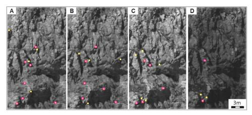
Figure 4.6. Points matched between digital images converted to grayscale and band 1: 1.336 $\mu$  (A), band 3: 1.346 $\mu$  (B), band 60: 1.624 $\mu$  (C) and band 240: 2.502 $\mu$  (D) of the hyperspectral scan. Points matched in more than one band marked in purple.
