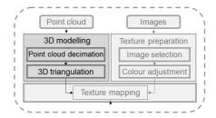
The result of the described above image- and laser-based surface reconstruction approaches is most commonly a point cloud and a set of images. The size of the dataset depends on the size of the outcrop and the density of the point cloud, but may be millions of 3D points and hundreds of digital images, covering hundreds of meters, or in the case of helicopter-based datasets, tens of kilometres of outcrop.
