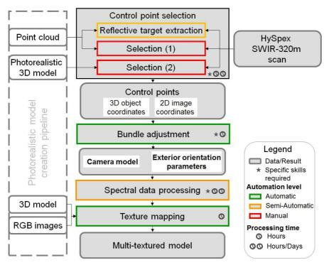
Figure 3.1. Workflow for integration of hyperspectral and lidar data, as described in (Kurz et al. 2011).
