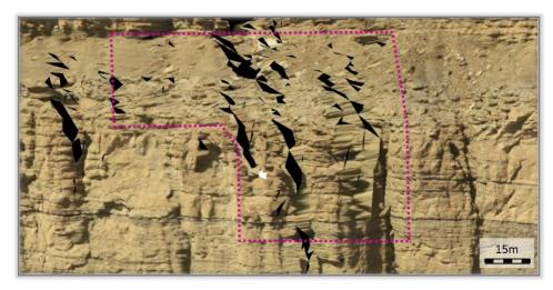
Figure 2.5. An example of a low quality (smeared) texture (marked in purple) resulting from poor image orientation with respect to the terrain model, indicating an image has been missed from those selected for texturing. Black areas denote mesh triangles without texture.
