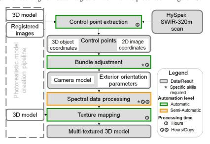
Figure 4.5. Workflow for semi-automatic integration of laser and image data with HySpex SWIR-320m imagery
