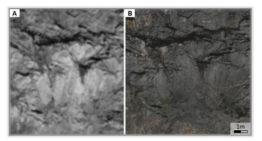
Figure 3.3. (A) Sample of a hyperspectral scan, band 1.336µm and (B) the corresponding area of the photorealistic model.
