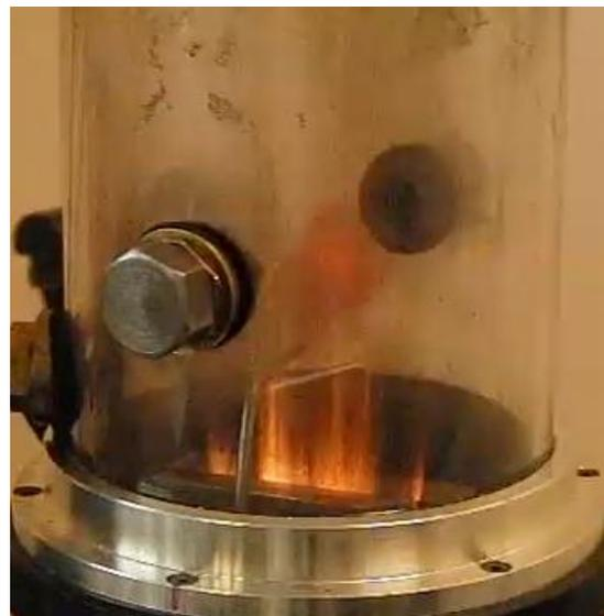
**Figure 4-4** High speed camera recording of second explosion test on rusted slit with gap opening 0.71 mm. No re-ignition.
