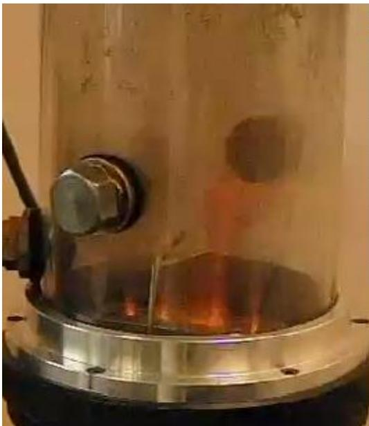
**Figure 4-3** High speed camera recording of first explosion test on rusted slit with gap opening 0.71 mm. No re-ignition.
