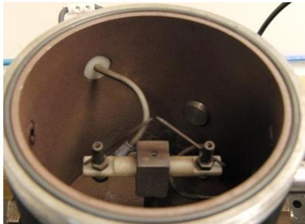
*Figure 3-9 Photograph of the adjustable ignition source located in the primary chamber.*
