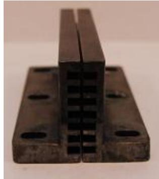
*Figure 3-4 Slits with crosswise grooves. Surface configuration PH-7.2.3.*
