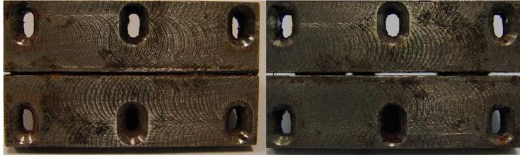
**Figure 4-2** Rusted slit at gap opening 0.72 mm before (to the left) and after (to the right) ten subsequent explosion tests.
