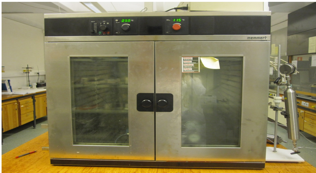
Figure 6.7 Core samples inside the heat cabin, cylinder to the right controls the confining pressure
