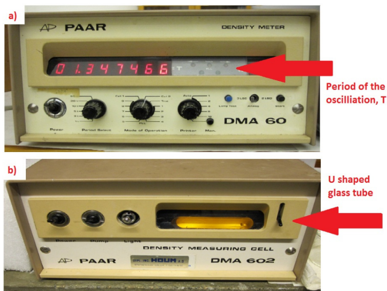
Figure 6.15 Densitometer: a) DMA 60 processing unit, b) DMA 602 HT density measuring cell
