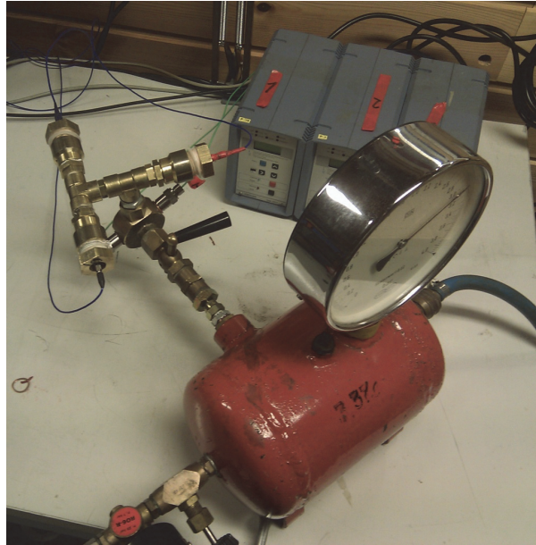
Figure 6.2 : Experimental setup for calibration of pressure transducers
