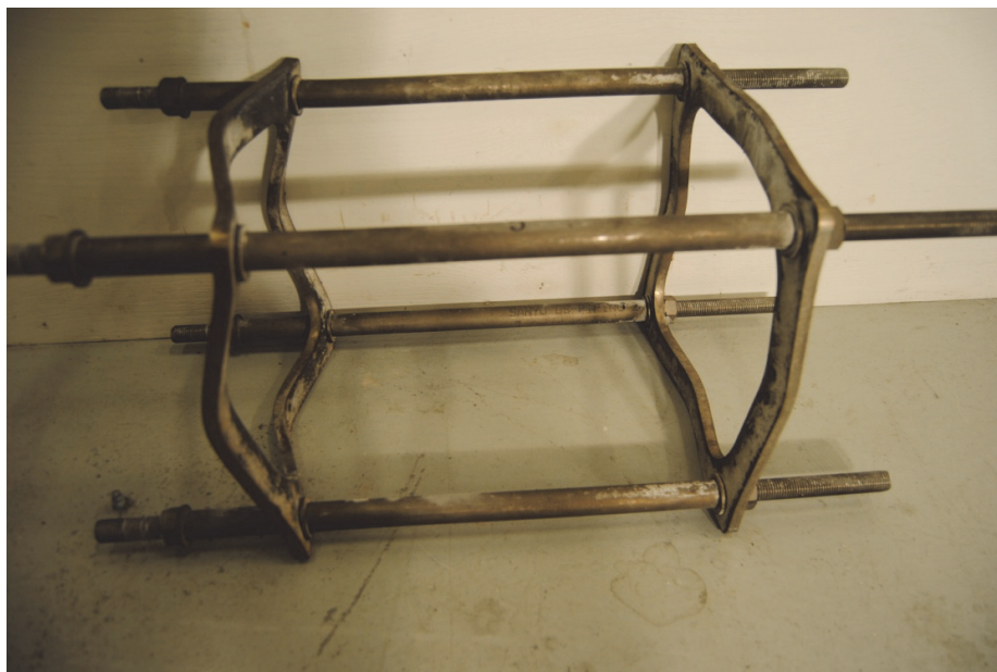
Figure 4.17 : Deformation to the last obstruction caused by high local overpressure in experiments with propane and obstacle configuration number 2(10 baffle plates). Flow direction from left to right, with the end wall 15 cm from the right baffle plate.
