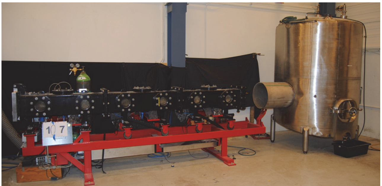
Figure 3.1 : The Flame Acceleration Tube and the dump tank
