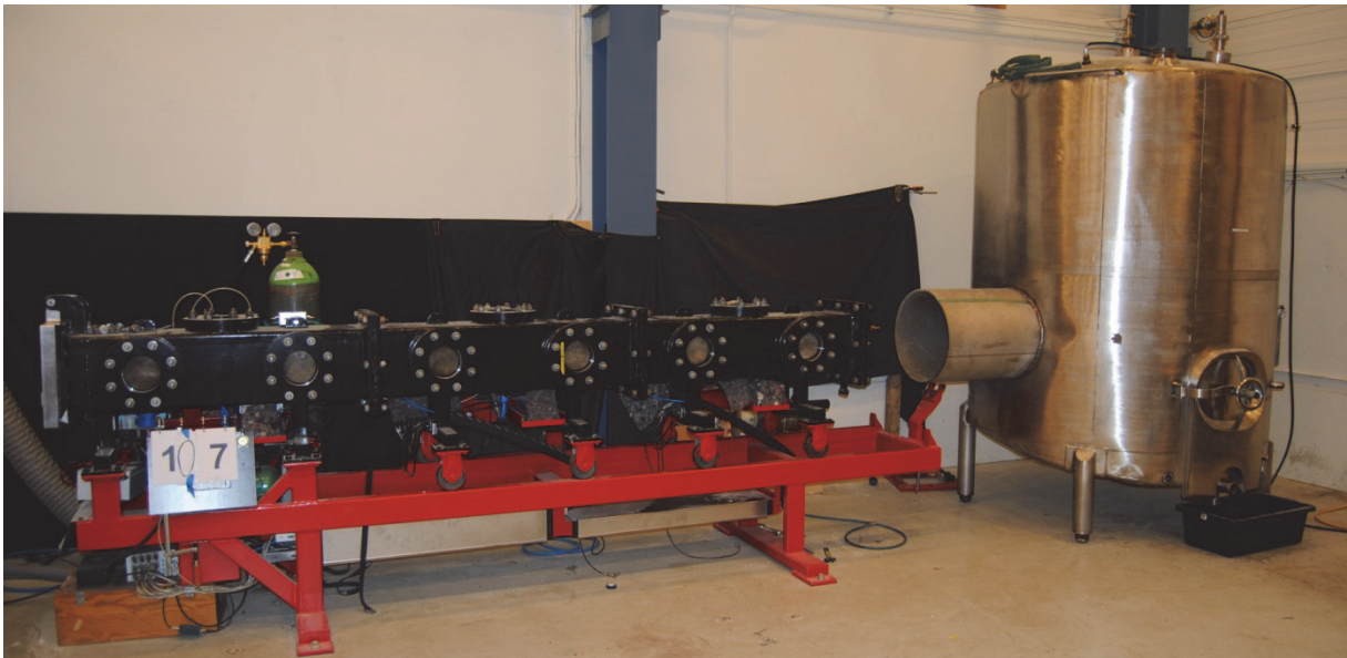
Figure 1.5 : The Flame Acceleration Tube and dump tank used in the experimental work
