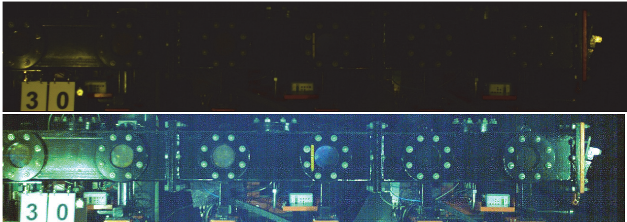
Figure 3.8 : Test nr. 30, 3.0% propane, flame at 94 ms after ignition, original and with image processing.
