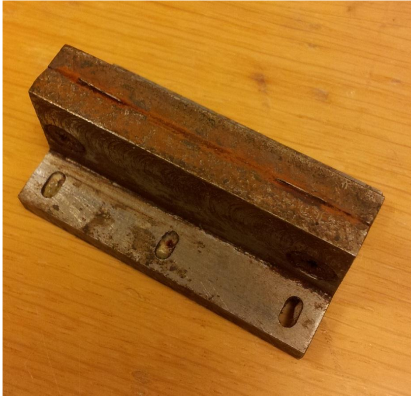
Figure 3.13 : One of the six slits that have been exposed to sea water for two months.
