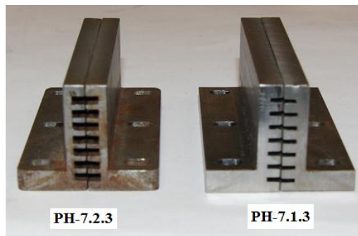
Figure 2.39 : Two different slit sets with multiple crosswise grooves with various widths. From (Solheim 2010).
