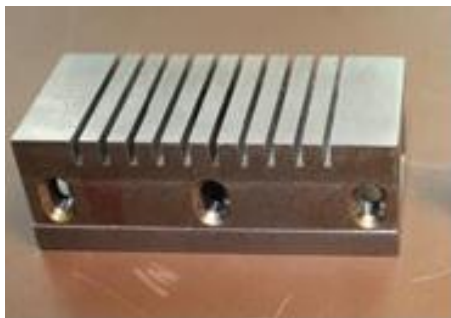
Figure 2.37 : Lengthwise and crosswise grooves respectively on the PRSA. From (Grosv 2010).
