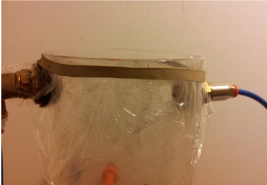
Figure 3.8 : Plastic foil used as the pressure relief during all experiments on the PRSA.
