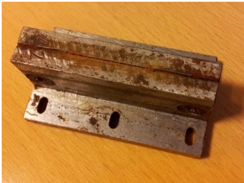
Figure 3.12 : One of the six slits that have been exposed to sea water for one month.
