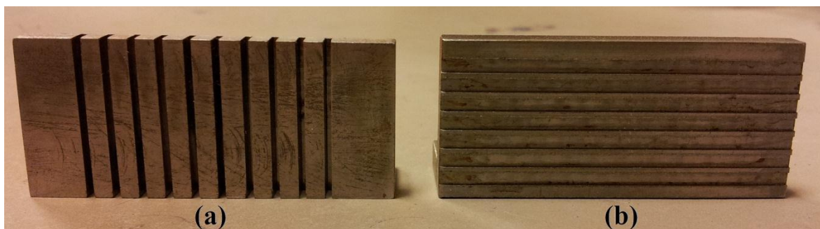
Figure 3.10 : (a) shows lengthwise grooves and (b) shows crosswise grooves.
