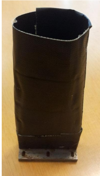
Figure 4.9 : The waterproof tube designed for testing the water flow ability through the flame gap opening.
