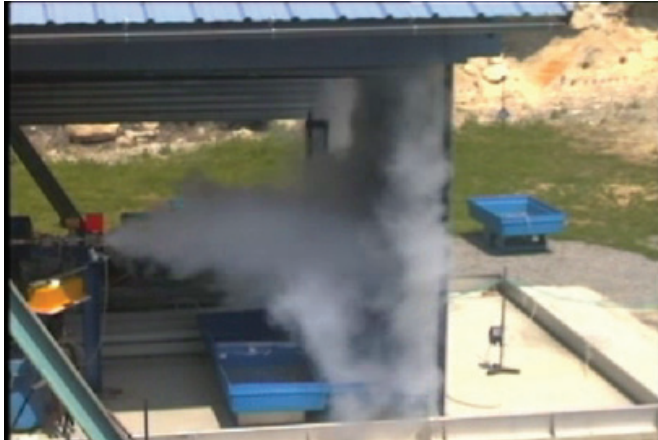
Figure 2.2: Photograph of an impinging propane release taken during one of the FLIE-INERIS tests (taken from Bonnet et al. (2005) ).
