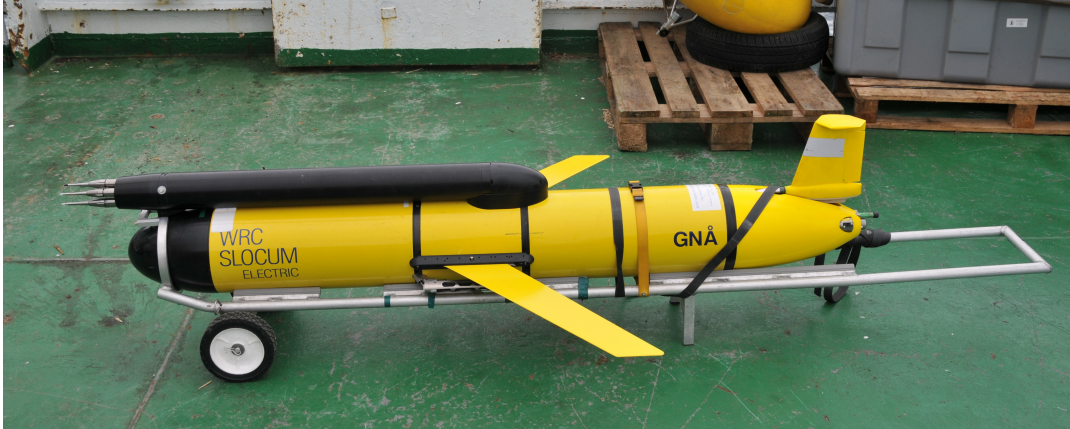
Figure 3.1: Slocum Electric glider Gná equipped with MicroRider package with microstructure sensors.
