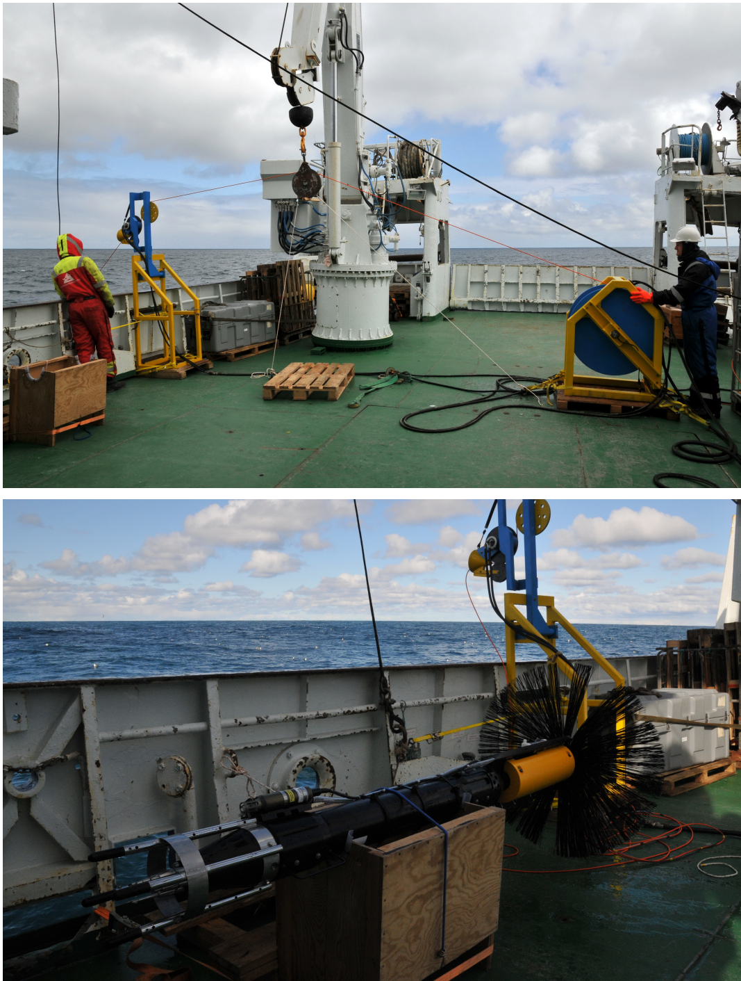
Figure 3.3: Top: The deck setup, with the winch to the right in the photograph, cable is fed to the linepuller to the left, mounted to the ship's railing. Bottom: The VMP lying on deck between deployments.
