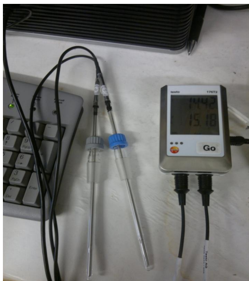
Figure 2.3: The Testo logger (Testo 176t2) with the sensor, used to control the temperature in the hydrate system.
