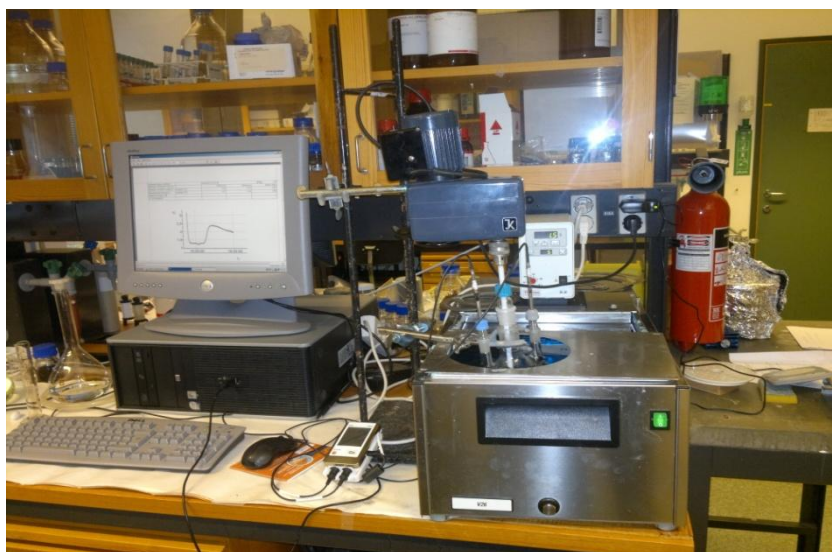
Figure 2.2: The experimental setup used for hydrate investigation.
