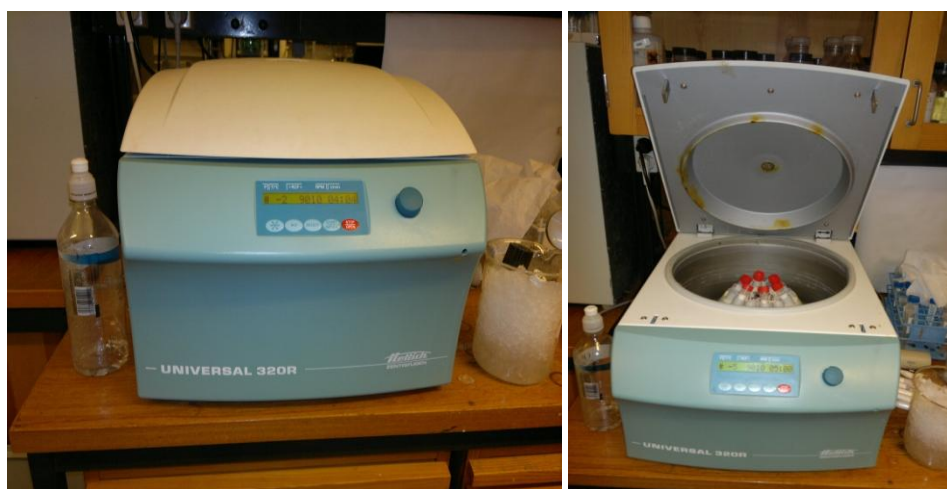
Figure 2.4: Universal 320 centrifuge use to separate the excess water.
