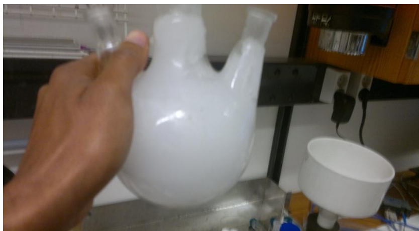
Figure 2.9: Illustrate the reactor (Three necks glass) with hydrate after forming.
