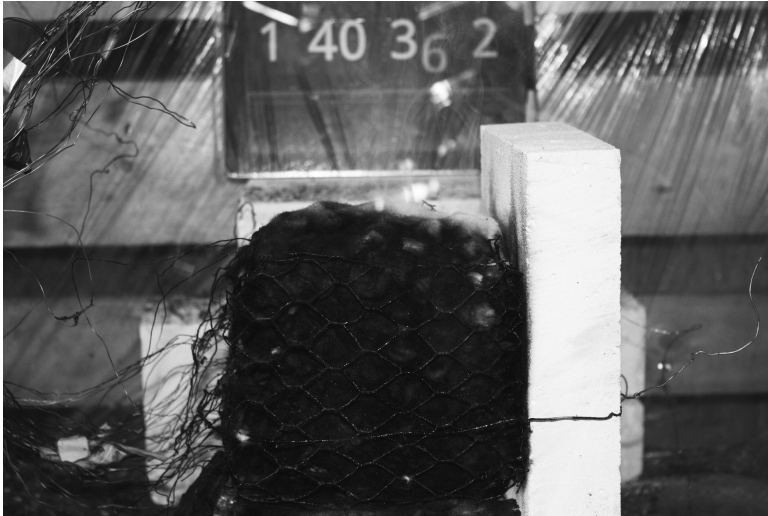
Figure 4.5: Photo of the cotton cube with density 60 \text{ kg/m}^3 at 100 minutes, 17 minutes before transition to flaming occurred. The smoldering front has consumed the outer part of the cotton sample. The temperature profile in the cotton is shown in figure 4.6a.
