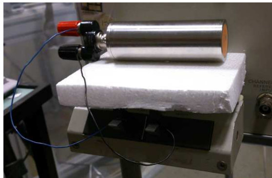
Figure 3.7: Electrical measurement setup for the piezoelectric transducers constructed during this work.
